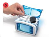
Grasp black ring retainer, and gently wrap tubing anticlockwise around rotor. Pull up retainer and insert into slot.
