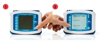
Locate power button on lower right hand corner of control
