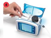
Grasp finger tab on valve and insert valve into valve slot on the left.
