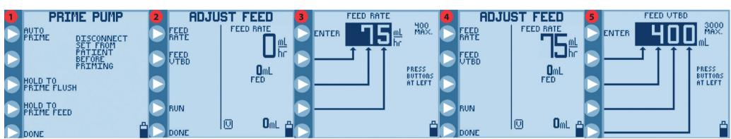
Press **PRIME PUMP** followed by **AUTO PRIME** to automatically prime or **HOLD TO PRIME** to manually prime both feed and flush lines.
